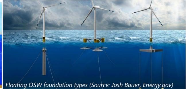
The depth of Maine’s coastal waters, which are routinely over 250 feet deep at distances of 10 nautical miles (nm) from the shoreline, rule out the economical use of fixed-bottom foundations.
